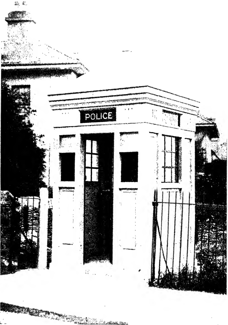
Fig. 1.—Precast Concrete Police Kiosk made with Limestone Aggregate.
